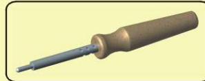
Soldering iron (40~50 watts) and a small amount of solder. ! Be careful on hot parts
