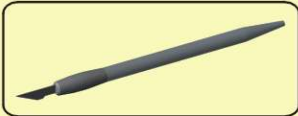
Hobby knife Use for trimming and cutting. ! This knife cuts plastic and fingers with equal ease, so be careful
